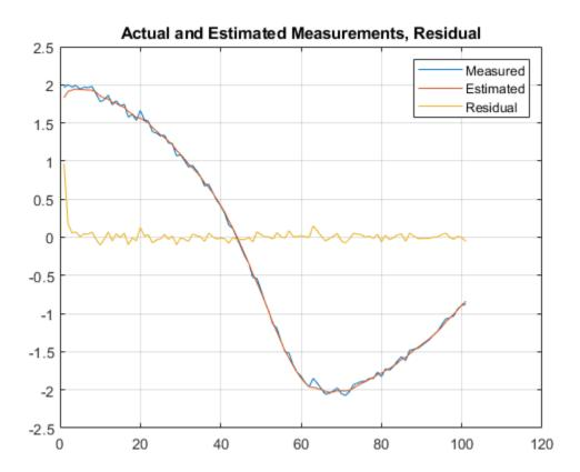
The estimate tracks the measurement closely. After the initial transient, the residual remains relatively small throughout the run.
