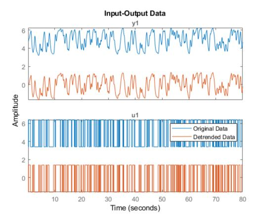
The detrended data has shifted by about 5 units. Inspect Tr to obtain the precise mean values that detrend computed and subtracted. These values are returned in the InputOffset and OutputOffset properties.
