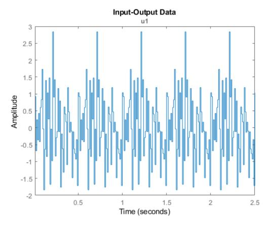
The plot shows that u contains a random segment of 50 samples, repeated 5 times. The signal is a Gaussian white noise signal with zero mean and variance one.
