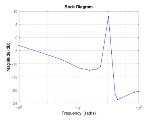
bodemag plots the frequency response at the specified frequencies only.
