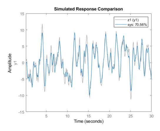
The plot illustrates the differences between the model response and the original data. The percentage shown in the legend is the NRMSE fitness value. It represents how close the predicted model output is to the data.
