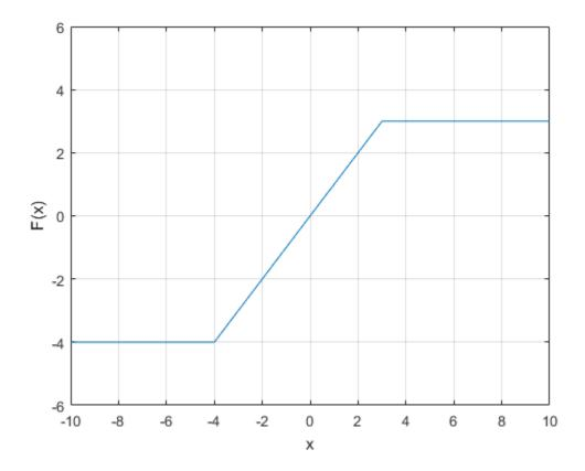
The value F(x) is computed by evaluate (NL, x), where NL is the saturation object.
