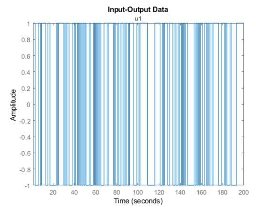
The generated signal is a random binary input signal with values -1 or 1. You can use the generated input signal to simulate the output of your system using the sim command.
