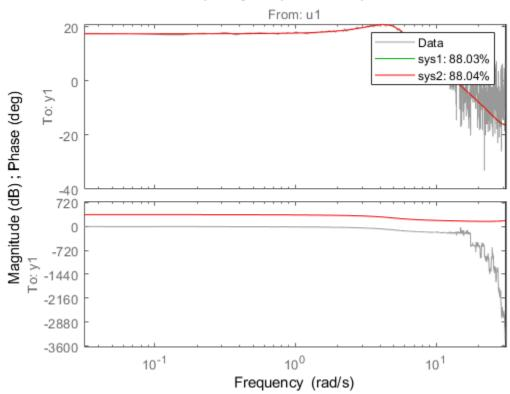
The two models have NRMSE fit values that are nearly equal with respect to the data from which they were calculated.
