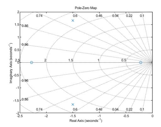
Turning on the grid displays lines of constant damping ratio (zeta) and lines of constant natural frequency (wn). This system has two real zeros, marked by o on the plot. The system also has a pair of complex poles, marked by x.
