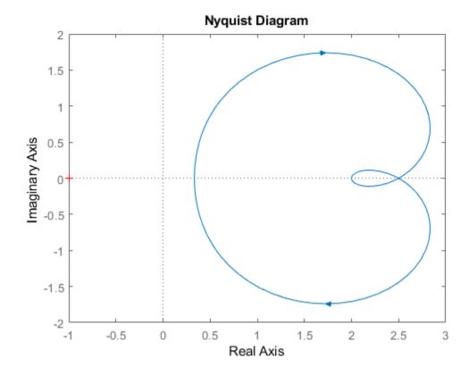
The nyquist function can display a grid of *M*-circles, which are the contours of constant closed-loop magnitude. *M*-circles are defined as the locus of complex numbers where the following quantity is a constant value across frequency.
