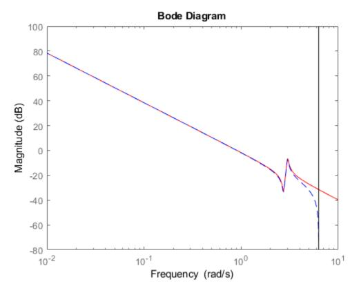
The first LineSpec argument 'r' specifies a solid red line for the response of H. The second LineSpec argument 'b--' specifies a dashed blue line for the response of Hd.
