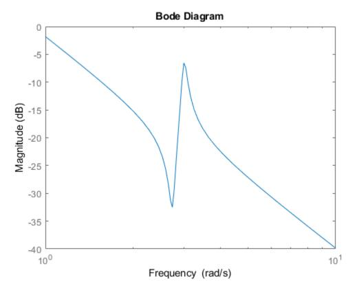
bodemag automatically selects the plot range based on the system dynamics.
