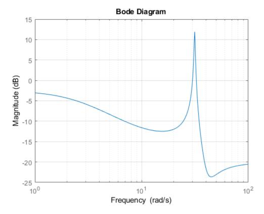
The cell array {1,100} specifies the minimum and maximum frequency values in the Bode magnitude plot. When you provide frequency bounds in this way, the function selects intermediate points for frequency response data.
