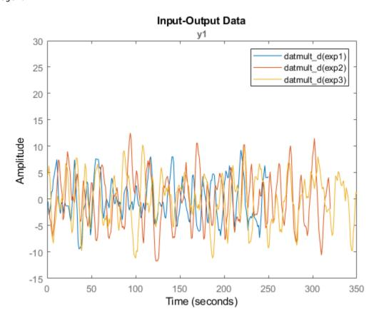
The experimental data are now better aligned, and do not drift significantly away from zero mean.
