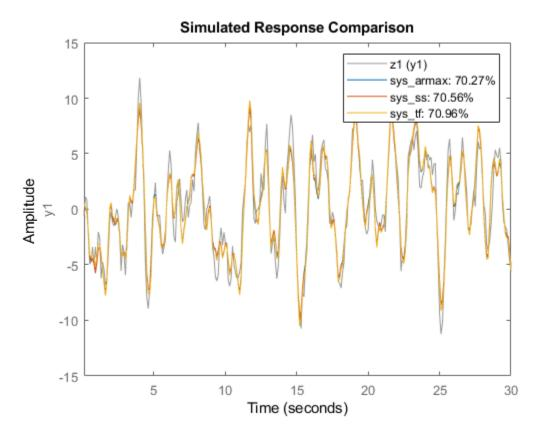
For this set of data, along with the default settings for all the models, the transfer-function form has the best NRMSE fit. However, the fits for all models are within about 1% of each other.
