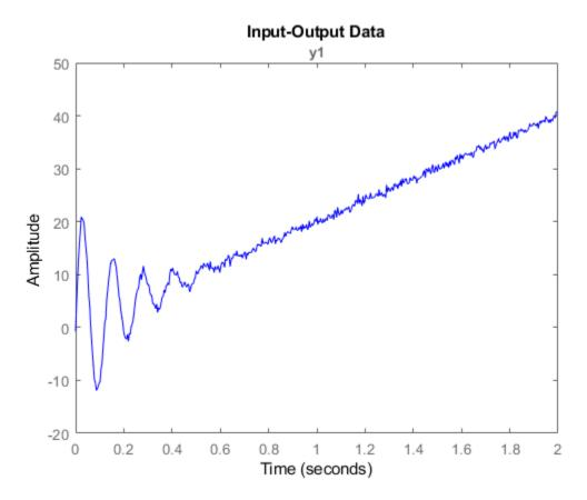
The plot shows a clear linear trend in the data. Use detrend linear option (Type = 1) to subtract the trend from the data. detrend fits the data and determines the linear trend to subtract. Include the TrendInfo object Tr as an output argument so you can see what detrend subtracts.
