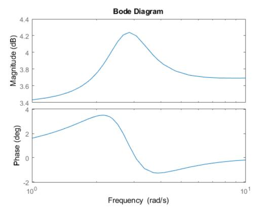
Change the units to Hz and suppress the phase plot. To do so, edit properties of the plot handle, h. setoptions(h,'FreqUnits','Hz','PhaseVisible','off');
