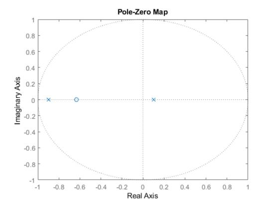
System poles are marked by x, and zeros are marked by o.
