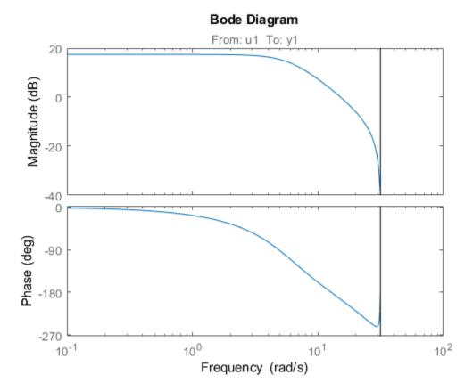
z1 is an iddata object that contains time domain system response data. sys is an idpoly model containing the identified polynomial model. h is the plot handle for the bode response plot of sys.
