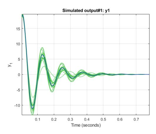
The blue line plots the simulated response of the original nominal model sys. The green lines plot the simulated response of the 20 perturbed realizations of sys.
