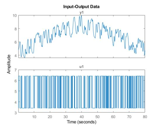
Both input and output plots show a bias. However, the output plot also shows an inverted V-shape trend that is not present in the input data.
