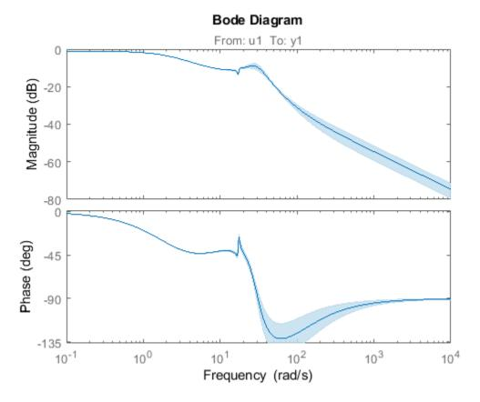
The plot shows the effect of the uncertainty in Plant on the closed-loop response.
