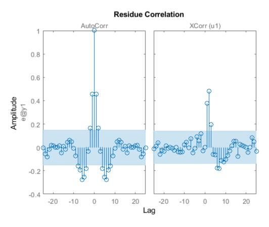
The correlations are calculated until the default maximum lag, 25. The 99% confidence region marking statistically insignificant correlations displays as a shaded region around the X-axis.
