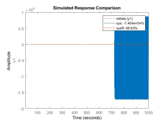
The large negative fit result for the unregularized model indicates a poor fit to the data. Estimating a regularized model produces a significantly better result.
