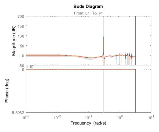
The regularized model m2 has a reduced variance compared to the unregularized model m1.
