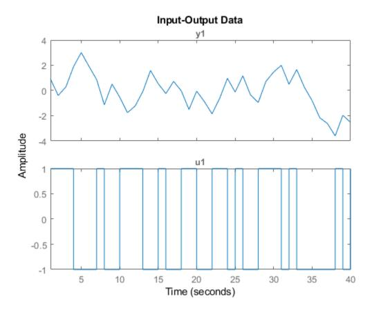
This data contains a change in time delay from 2 to 1, which is difficult to detect by examining the data.
