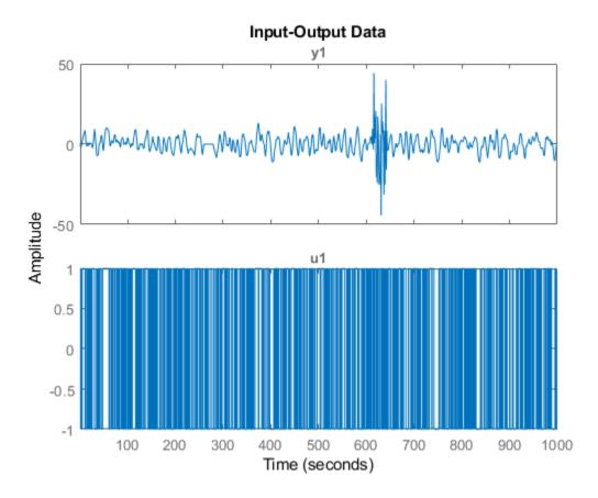
Bad portions of data are detected around sample 250 to 280 and between samples 600 to 650. Cut out these bad portions to form a multiple-experiment data set and merge the data.
