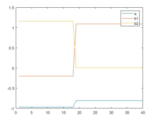
The data has been divided into two segments, as indicated by the change in model parameters around sample number 19. The increase in b1, along with a corresponding decrease in b2, shows the change in model delay.
