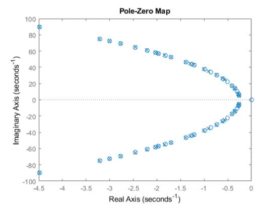
From the plot, observe that there are numerous near-canceling pole-zero pairs that could be potentially eliminated to simplify the model, with no effect on the overall model response. pzmap is useful to visually identify such near-canceling pole-zero pairs to perform pole-zero simplification.
