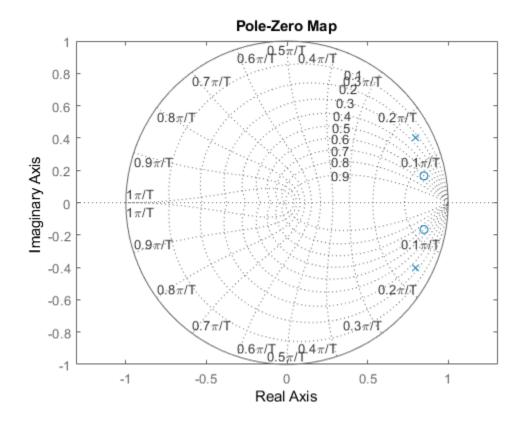
Observe that the frequencies on the z-plane grid are normalized in terms of  $f\frac{\pi}{T}$ . To obtain the true frequency values on the grid, specify the sample time with the zgrid command.
