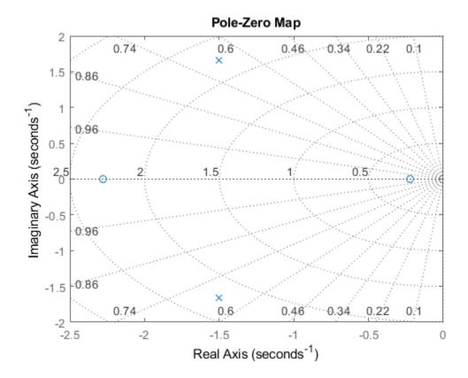
Turning on the grid displays lines of constant damping ratio (zeta) and lines of constant natural frequency (wn). This system has two real zeros, marked by o on the plot. The system also has a pair of complex poles, marked by x.
