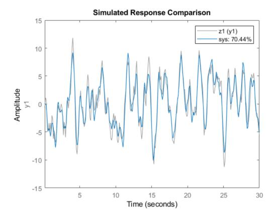
The plot shows that the fit percentage between the simulated model and the estimation data is greater than 70%.
