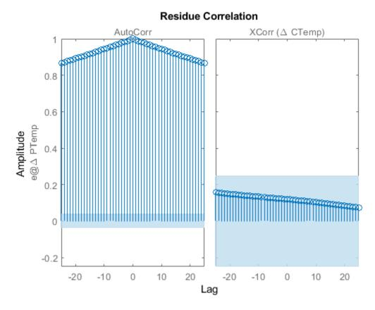
The figure shows that the residuals are correlated. To account for that, add a first order ARMA disturbance component to the process model.
