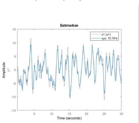
Execute the task from the **Live Editor** tab using **Run**. A plot displays the estimation data, the estimated model output, and the fit percentage.
