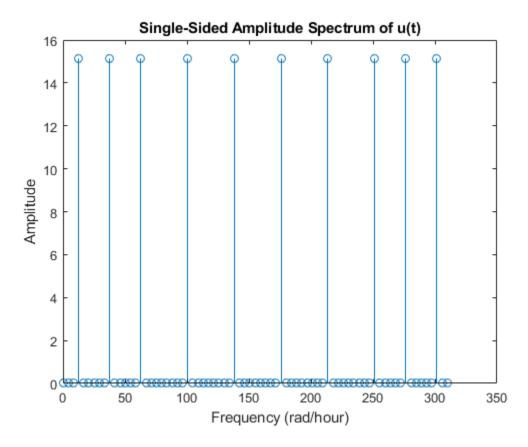
The generated plot shows the frequencies of the 10 sine waves used to generate the signal. For example, the plot shows that the first sine wave has a frequency of 12.57 rad/hour, the same as freq(1).
