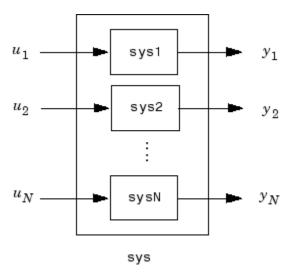
For systems with transfer functions  $H_1(s)$ , . . . ,  $H_N(s)$ , the resulting system sys has the block-diagonal transfer function
