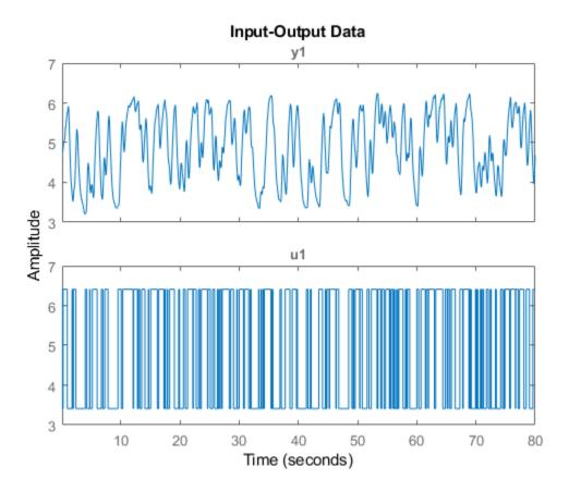
The known offset of 4 (from operating point 1) is visible in the plots. You can construct a TrendInfo object to capture this offset, using the function getTrend.
