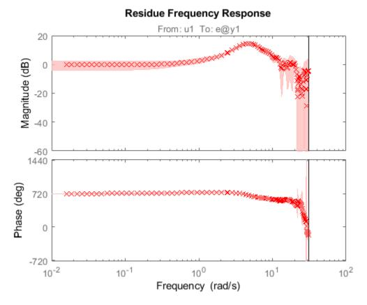
For frequency-domain data, resid plots the Bode plot showing frequency response from the input to the residuals.
