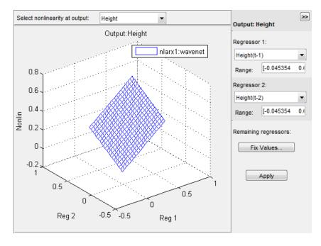
To understand what is plotted, suppose that  $\{r1, r2, ..., rN\}$  are the N regressors used by a nonlinear ARX model M with nonlinearity nl corresponding to a model output. You can use getreg(M) to view these regressors. The expression Nonlin = evaluate(nl, [v1, v2, ..., vN]) returns the model
