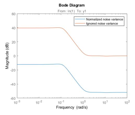
The difference between the bode magnitudes of the  $noise\_model\_innovation$  and  $noise\_model\_normalized$  is approximately 51 dB. As expected, the magnitude difference is approximately equal to 20\*log10(L).
