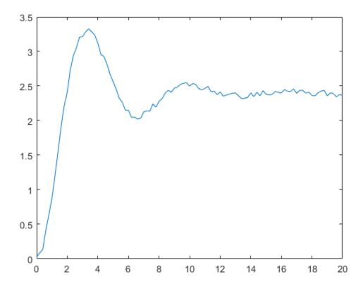
Compute step-response characteristics from this response data using stepinfo. If you do not specify the steady-state response value yfinal, then stepinfo assumes that the last value in the response vector y is the steady-state response. Because there is some noise in the data, the last value in y is likely not the true steady-state response value. When you know what the steady-state value should be, you can provide it to stepinfo. For this example, suppose that the steady-state response is 2.4.
