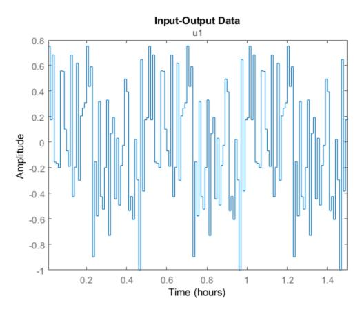
The signal u is generated using 10 sinusoids and has a period of 0.5 hours and 3 periods.
