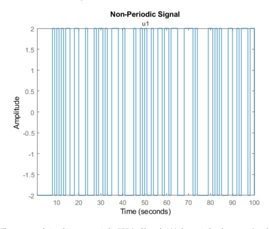
The generated signal is a nonperiodic PRBS of length 100 that switches between -2 and 2.
