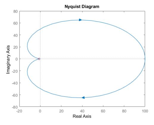
Zoom in on the critical point, (-1,0). You can do so interactively by right-clicking on the plot and selecting **Zoom on (-1,0)**. Alternatively, use the **zoomcp** command on the plot handle h.
