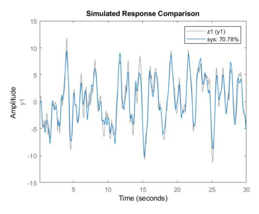
The plot shows that the fit percentage between the simulated model and the estimation data is greater than 70%.
