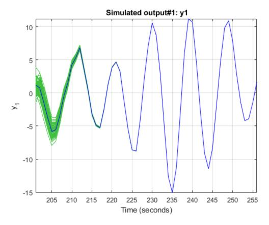
The blue line plots the simulated response of the original nominal model sys. The green lines plot the simulated response of the 100 perturbed realizations of sys. The software uses a different realization of the initial states to simulate each perturbed model. Initial states are drawn from a Gaussian distribution with mean InitialCondition and covariance X0Covariance.
