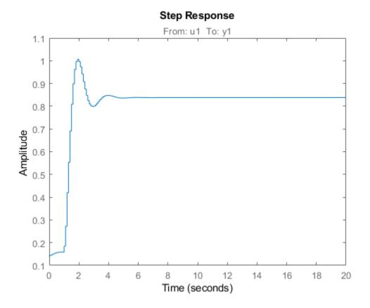
The step response is a steady-state value of 0.8383 at T = 20 seconds.
