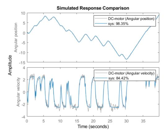
sys provides a 98.35% fit for the angular position and an 84.42% fit for the angular velocity.
