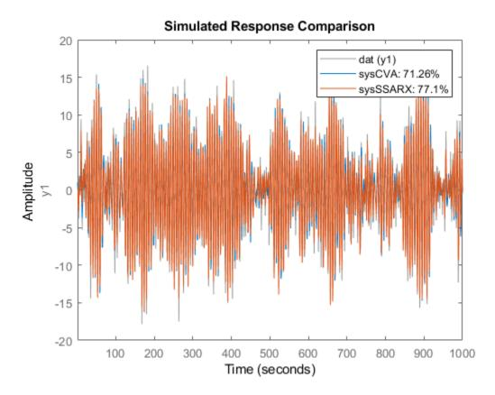
As the plot shows, the model estimated using the SSARX algorithm produces a better fit than the model estimated using the CVA algorithm.
