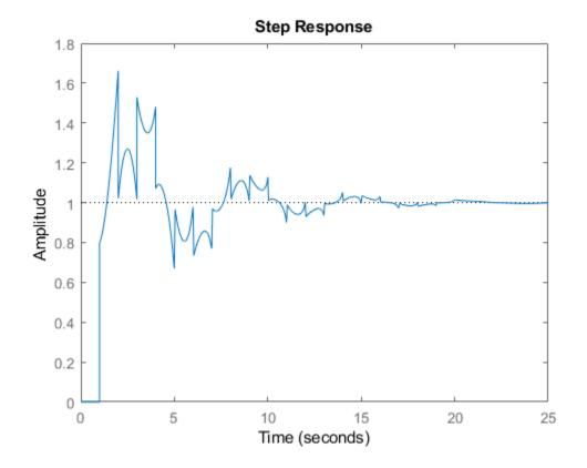
The system step response displayed is chaotic. The step response of systems with internal delays may exhibit odd behavior, such as recurring jumps. Such behavior is a feature of the system and not software anomalies.
