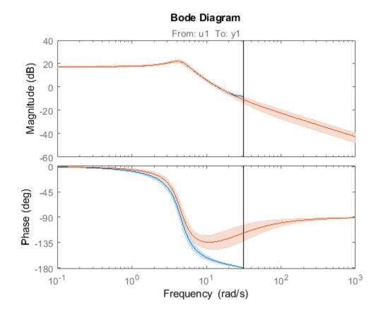
The uncertainties of sys1c and sysd are comparable up to the Nyquist frequency. However, sys1c exhibits large uncertainty in the frequency range for which the estimation data does not provide any information.
